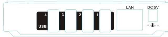
DC Power Jack: Socket for DC Power Plug 5V, 2A
